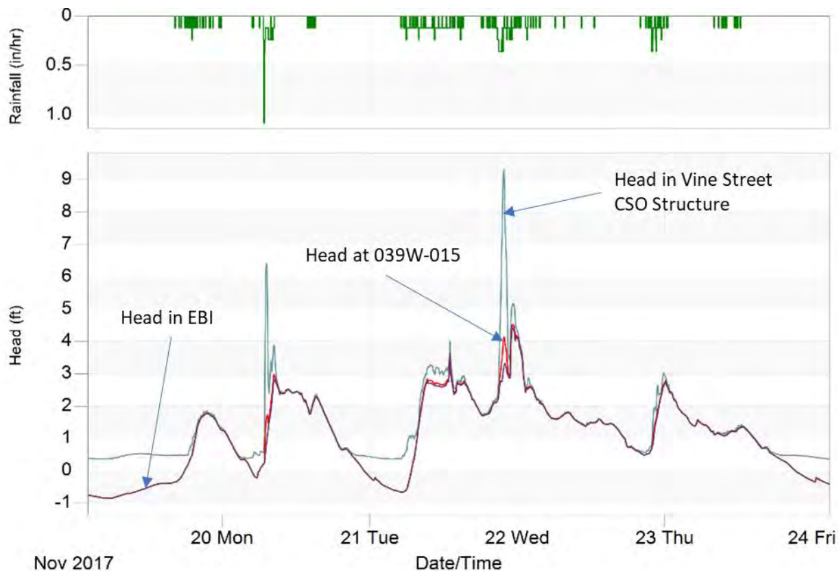
Figure 7-1: Head at 039W-015 (red), Head in the EBI Near the Denny Lake Union Regulator (blue), and Head in the Vine Street CSO Structure (turquoise)
