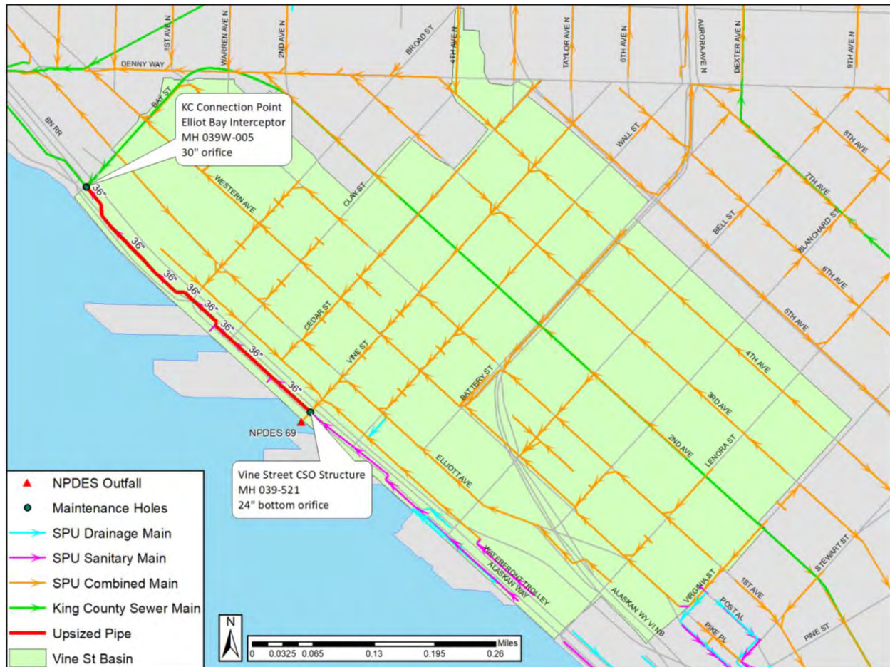
Figure 9-1: Flow Transfer Option A
